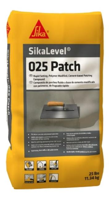
SikaLevel®-025 Patch is a fast drying, self-curing, polymer-modified, cement-based patching compound that rapidly develops high compressive strength. Use for smoothing, leveling, patching, and filling cracks, holes and voids in concrete and approved wood underlayments prior to the installation of floor coverings. From featheredge to ½" floor coverings can be installed 1 hour after application.
