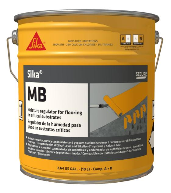
Sika MB is a 2-component, solvent free, low viscosity, epoxy for use under flooring products, self-leveling underlayment's, floating floors and other flooring systems that require protection from subfloor moisture.
