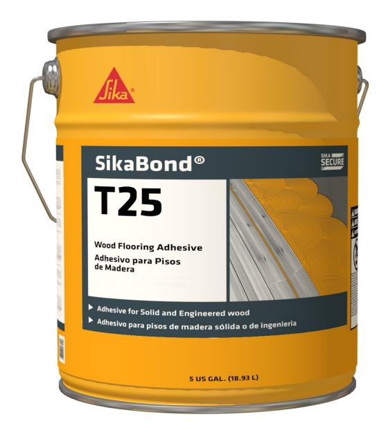
SikaBond T25 is a one-component, low odor, moisture cured polyurethane adhesive for full surface bonding of wood flooring and rubber flooring. SikaBond T25 will tenaciously bond wood to most surfaces, including concrete, plywood, and self-leveling and patch underlayment's that have been properly prepared.
